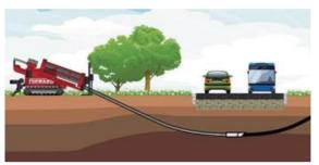
Once the appropriate permits have been issued, the operator establishes an entry and exit point and then, often with the use of bentonite, drills the borehole following a designed path under the surface. The bore is then reamed to the necessary diameter before the new pipe is pulled through the hole and connected with the line.
