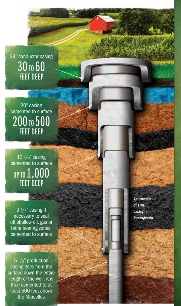
PENNSYLVANIA DEPARTMENT OF ENVIRONMENTAL **PROTECTION** REGULATIONS INCLUDE STRINGENT QUALITY AND MONITORING REQUIREMENTS FOR STEEL CASING AND CEMENT TO **ENSURE THAT FRESH GROUNDWATER ZONES ARE** PROTECTED.
